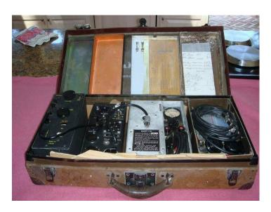
This unit was similar to other suitcase spy radio sets developed by various European countries during WW2. Its crystal controlled transmitter provided a CW output of about 8-15 watts.
