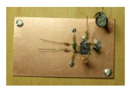
When we apply 6 volts between the positive supply and ground, and we connect headphones or a small speaker to the audio output, and touch an input pin, we should hear a buzzing sound, indicating that the circuit is working. Good. Now we can move on.
