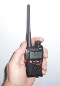
another member of the software defined radio offerings now flooding the amateur radio marketplace. It uses a 3.8 volt cellphone battery, and each charge with intermittent transmit should last around 4-6 hours, making it an ideal candidate for repeater operations via a cross-band mobile rig at public service events.
