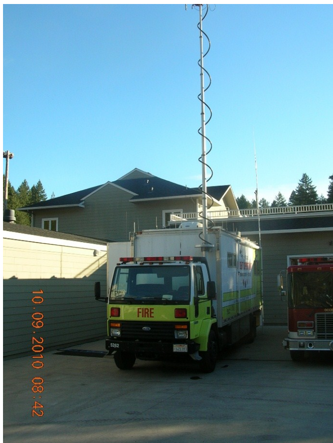
(Left) The County Communication Van with KQ6OB's J-pole mounted at the left rear.
