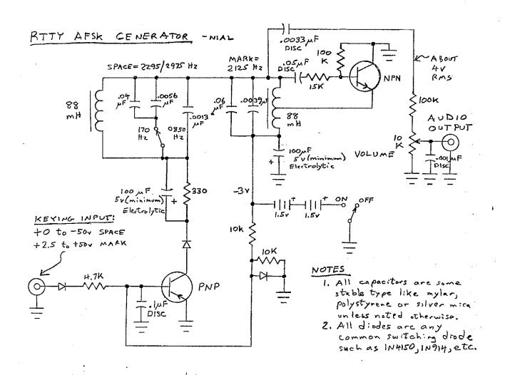
If you have easy access to a pair of 88mH toroids, here's a simple, 2 transistor audio frequency-shift keyer you can build. It's basically a Hartley Oscillator operating at Audio Frequency. The transistors can be practically any small audio transistors you have in the junk box. If your keying voltage is of opposite polarity to that shown, just swap the NPN and PNP transistors, reverse the polarity of all three diodes and the two 100µF capacitors, and reverse the battery polarity.
